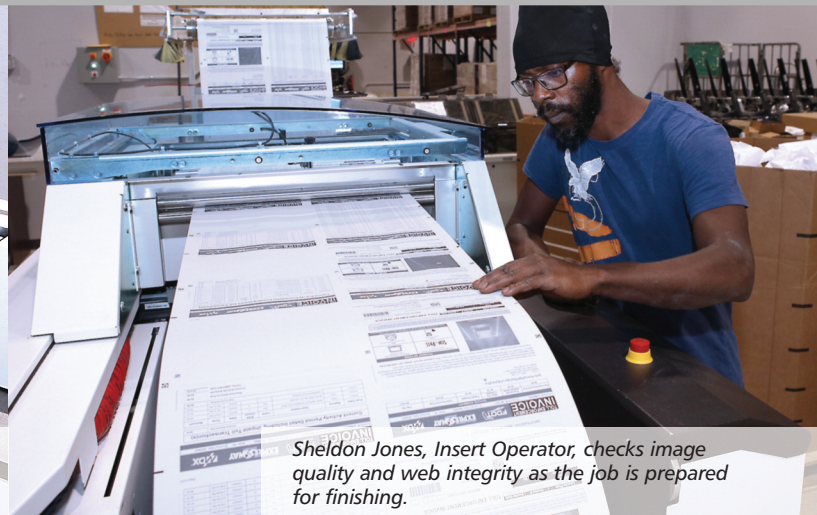
The new Hunkeler line includes the WM8 Web Merger which allows slitting and merging left under right or right under left.
